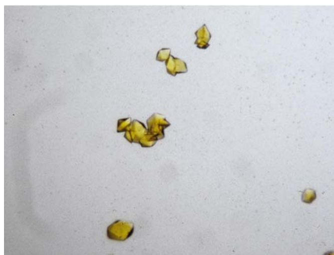
Figure 4 Crystals of 4 F1 5 F1 human fibronectin module pair after soaking overnight in 10 mM platinum (II) terpyridine chloride dihydrate. The crystals have changed from colourless to orange.
